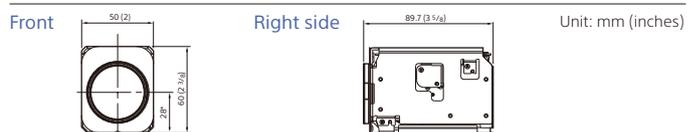
\* The lens position is shifted down by approx. 2 mm than FCB-EV7520 series.
